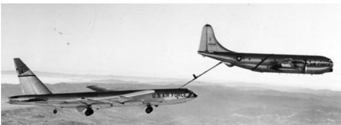
A Boeing B-52 Stratofortress refuels in flight from a Boeing KC-97 Stratotanker. The KC-97 had to enter a shallow dive to increase its speed, while the B-52 flew in landing configuration to fly slow enough to stay with the tanker. (U.S. Air Force)
