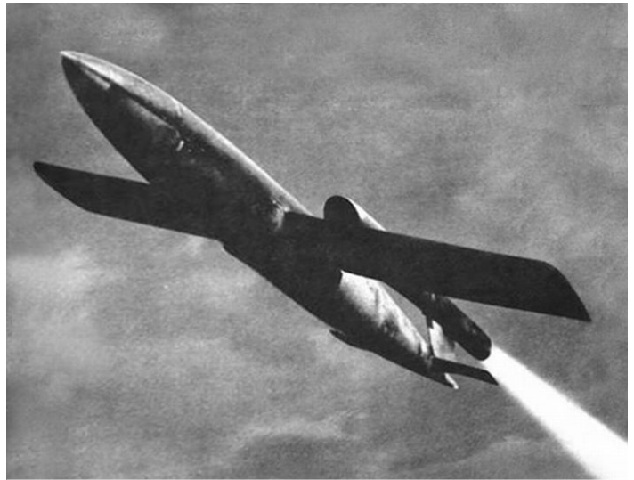
The V1 Flying bomb was an unmanned gyro guided plane that delivered a ton of high explosive each time one hurtled into the ground. 2419 were to explode in London between June 1944 and March 1945.
